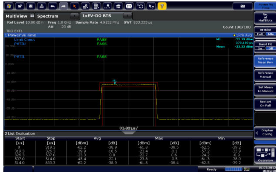
Fig. 3-21: Power vs Time measurement results in the 1xEV-DO BTS application
